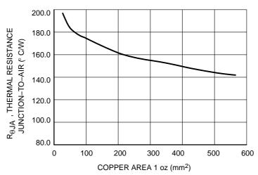
Figure 4. SOP-8 Thermal Resistance versus P.C.B. Copper Area
