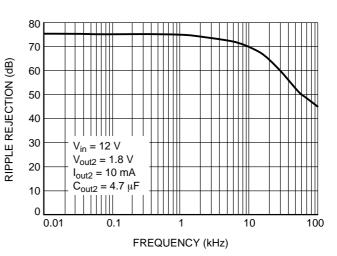
Figure 11. V<sub>out2</sub> Ripple Rejection
