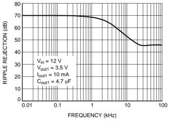
Figure 10. Vout1 Ripple Rejection
