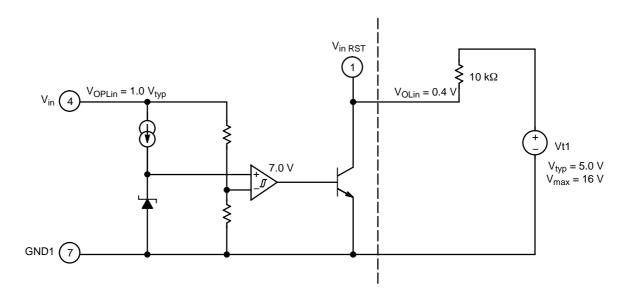
Figure 3. Threshold Operating Voltage  $V_{OPLin}$  Under Condition  $V_{OLin} = 0.4 \text{ V}$
