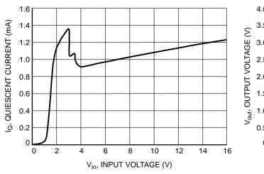
Figure 5. Quiescent Current versus Input Voltage
