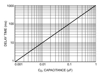
Figure 7. Delay Time versus Capacitance
