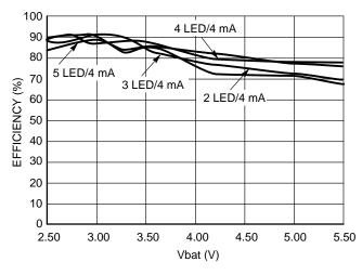
Figure 10. Overall Efficiency vs. Power Supply –  $I_{out}$  = 4.0 mA, L = 22  $\mu H$
