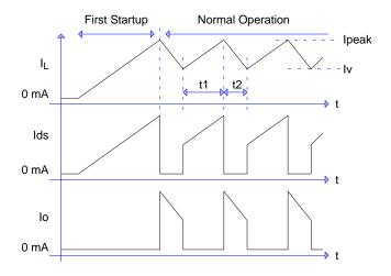
Figure 4. Basic DC-DC Operation
