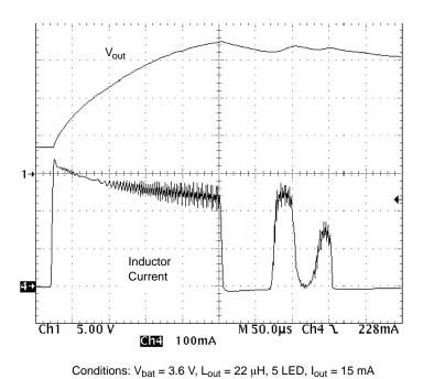
Figure 24. Typical Startup Inductor Current and Output Voltage
