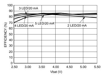
Figure 13. Overall Efficiency vs. Power Supply –  $I_{out}$  = 20 mA, L = 22  $\mu$ H
