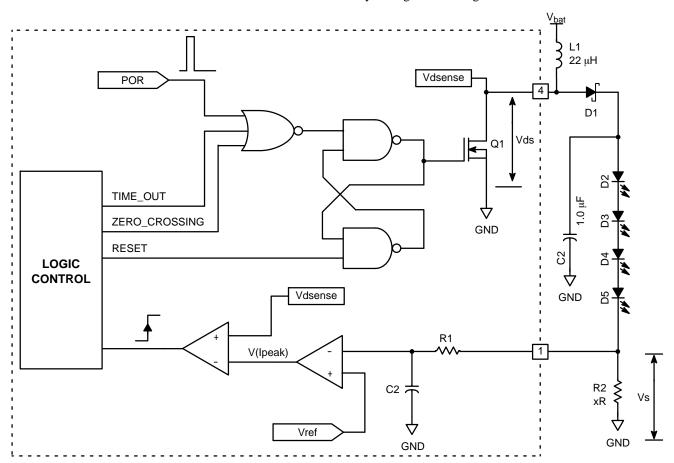
Figure 3. Basic DC-DC Converter Structure
