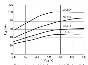
Test conditions: L = 22  $\mu$ H, Rsense = 2.0  $\Omega$ , Tamb = +25°C
