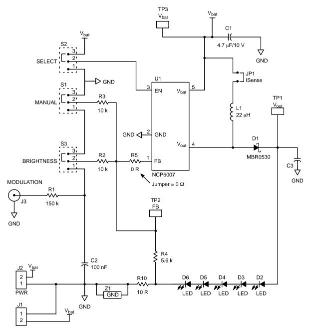
Figure 32. NCP5007 Demo Board Schematic Diagram
