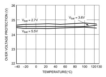
Figure 22. Overvoltage Protection
