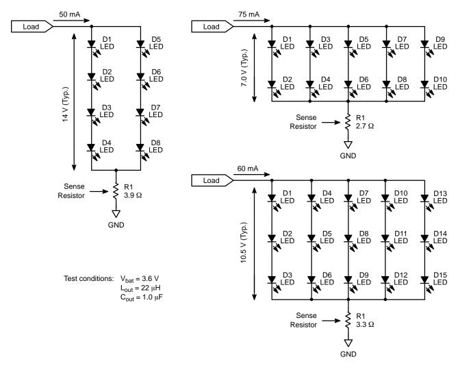
Figure 31. Examples of Possible LED Arrangements
