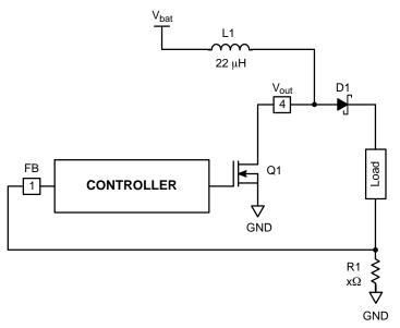
**Figure 8. Output Current Feedback**
