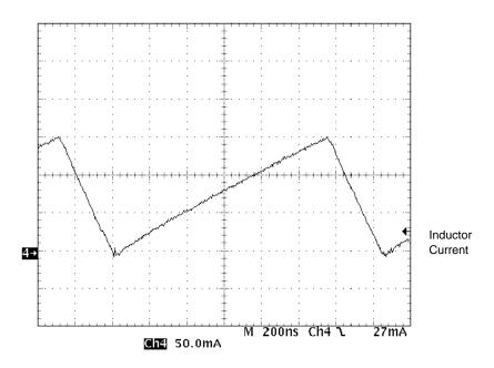
Conditions:  $V_{bat}$  = 3.6 V,  $L_{out}$  = 22  $\mu\text{H}, \, 5$  LED,  $I_{out}$  = 15 mA
