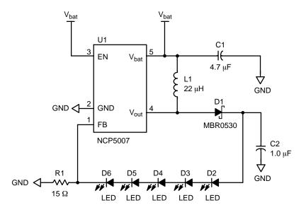
Figure 28. Basic DC Current Mode Operation with Analog Feedback
