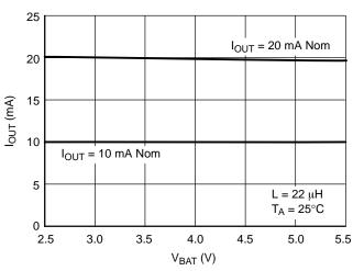
Figure 16. Current Variation vs. Power Supply with 4 Series LED's
