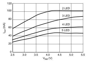
Test conditions: L = 22  $\mu$ H, Rsense = 2.0  $\Omega$ , Tamb = +25 $^{\circ}$ C
