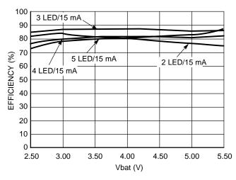
Figure 12. Overall Efficiency vs. Power Supply –  $I_{out}$  = 15 mA, L = 22  $\mu$ H
