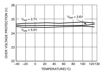
Figure 22. Overvoltage Protection
