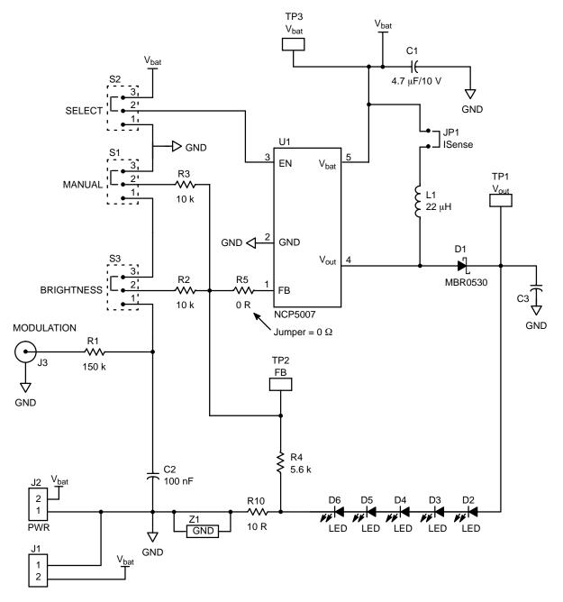
Figure 32. NCP5007 Demo Board Schematic Diagram
