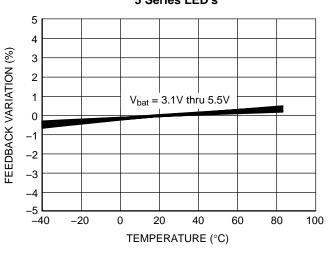
Figure 18. Feedback Voltage Stability
