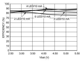
Figure 11. Overall Efficiency vs. Power Supply –  $I_{out} = 10 \text{ mA}, L = 22 \mu\text{H}$
