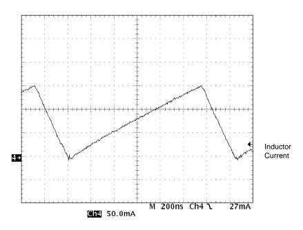
Conditions:  $V_{bat}$  = 3.6 V,  $L_{out}$  = 22  $\mu\text{H},$  5 LED,  $I_{out}$  = 15 mA
