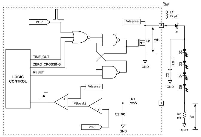
Figure 3. Basic DC-DC Converter Structure
