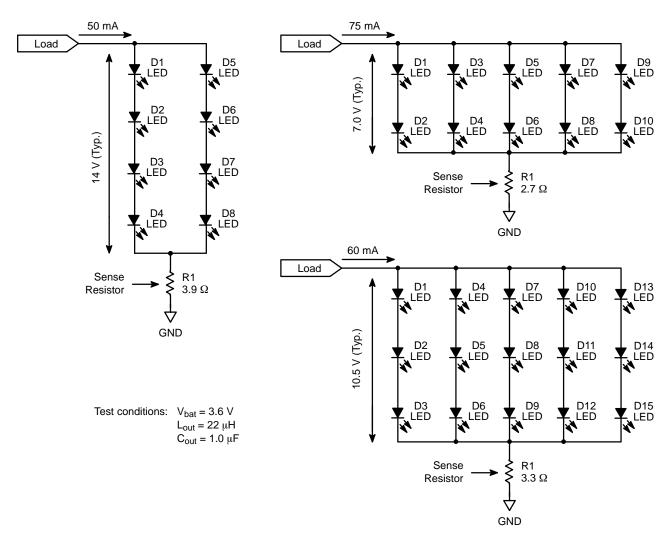
Figure 31. Examples of Possible LED Arrangements
