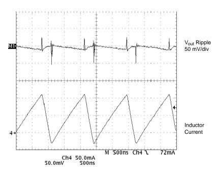
Conditions:  $V_{bat}$  = 3.6 V,  $L_{out}$  = 22  $\mu$ H, 5 LED,  $I_{out}$  = 15 mA
