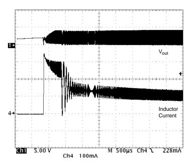
Conditions:  $V_{bat}$  = 3.6 V,  $L_{out}$  = 22  $\mu H,\, 5$  LED,  $I_{out}$  = 15 mA
