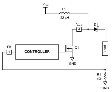
Figure 8. Output Current Feedback
