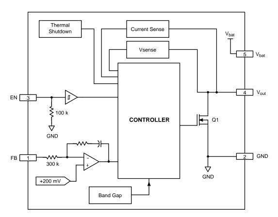
Figure 2. Block Diagram
