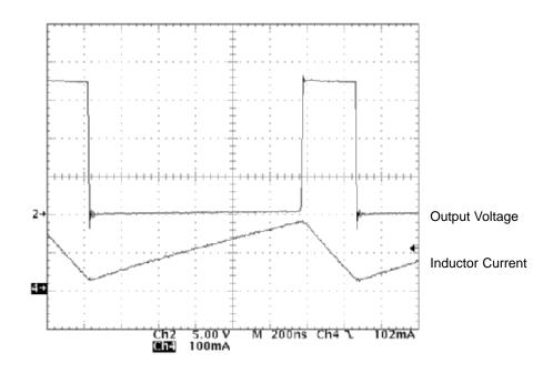
Test Conditions: L = 22  $\mu$ H, I $_{out}$  = 15 mA, V $_{bat}$  = 3.6 V, Ambient Temperature, LED = 5
