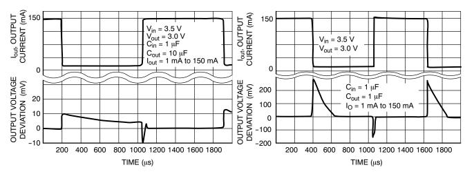
Figure 11. Load Transient Response
