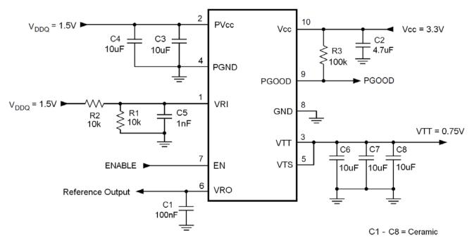
Figure 1. Typical DDR-3 Application Schematic
