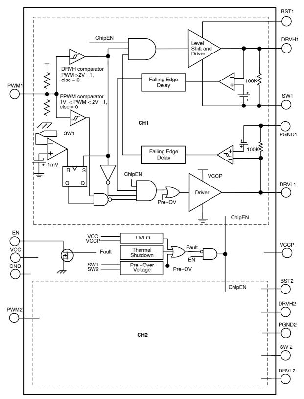
Figure 1. Internal Block Diagram and Typical Application
