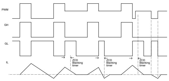
**Figure 4. Zero Current Detection**
