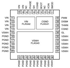
Figure 3. Pin Connections (Top View)
