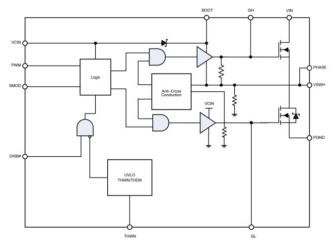
Figure 2. Simplified Block Diagram
