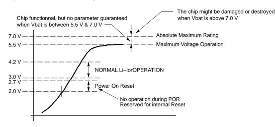
Figure 3. Understanding Integrated Circuit Voltage Limitations
