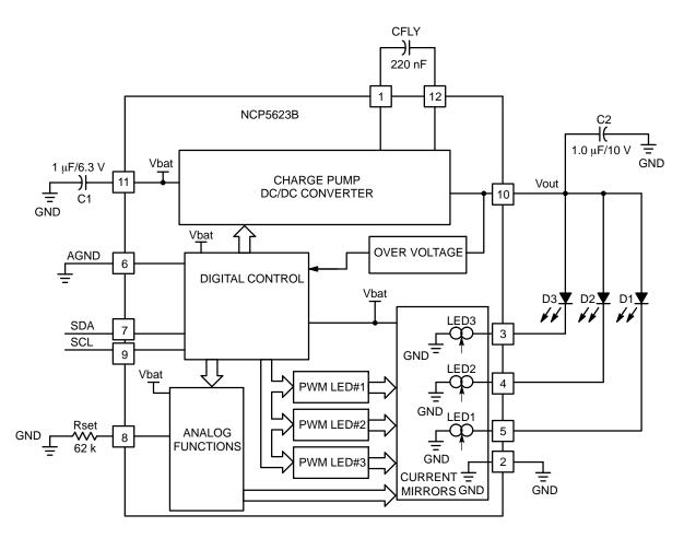
Figure 2. Simplified Block Diagram
