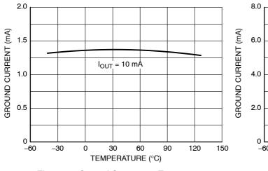
Figure 10. Ground Current vs. Temperature
