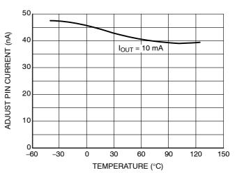
Figure 17. Adjust Pin Current vs. Temperature
