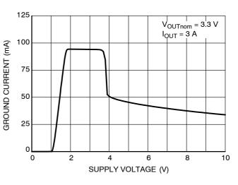
Figure 8. Ground Current vs. Supply Voltage
