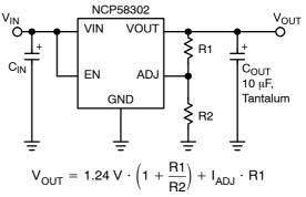
Figure 18. Adjustable Voltage Operation
