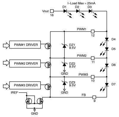
Figure 18. Basic PWM Internal Voltage Clamps
