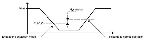
Figure 22. Undervoltage Lockout Basic Mechanism
