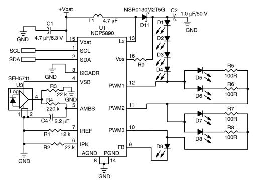
Figure 20. Paralleling Extension LED
