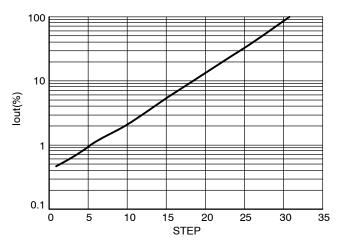
Figure 10. Typical lout (%) versus ILED Step Value
