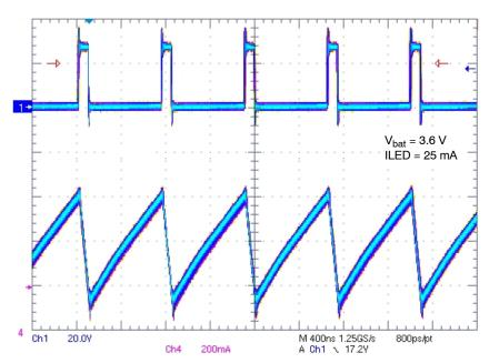
Figure 5. Typical Switching Operation
