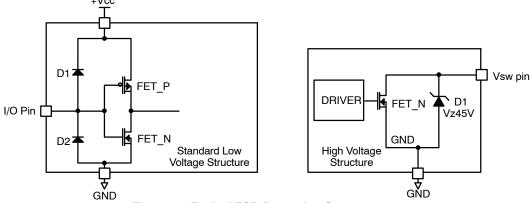
Figure 21. Typical ESD Protection Structures
