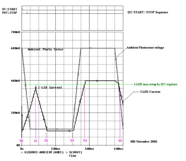
Figure 16. Basic Ambient Photo Sense Regulation (PSPICE simulation)
