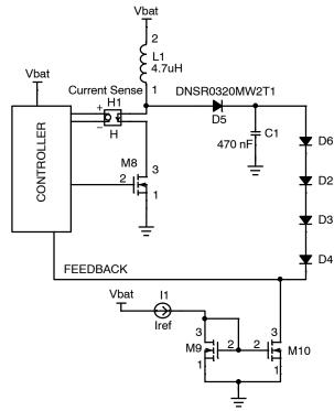
Figure 4. Simplified Boost Structure
