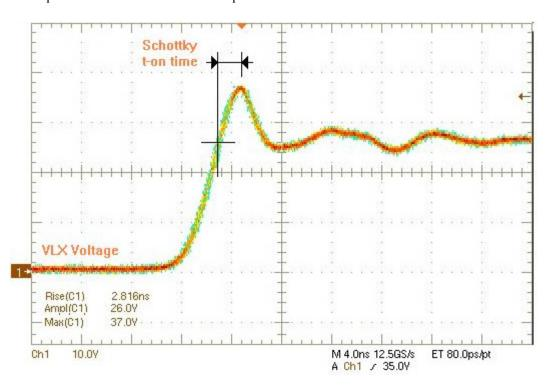
Figure 6. Typical Turn On Time of the Schottky Rectifier
