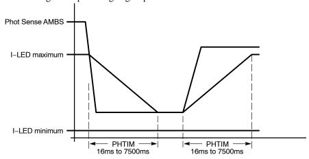
Figure 14. Basic Photo Sense Timing
