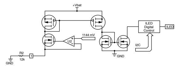
Figure 9. Basic Reference Current Source
