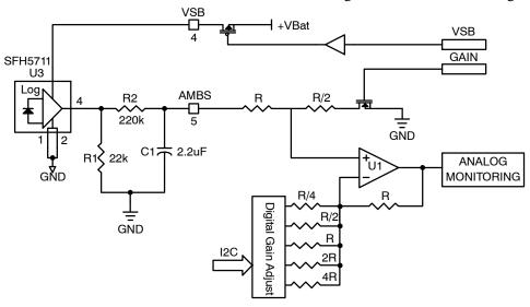
Figure 13. Basic Photo Sense Input Circuit
