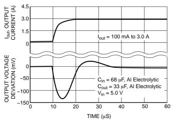
Figure 12. Load Transient
