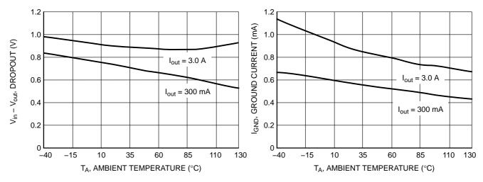
Figure 5. Dropout Voltage vs. Temperature
