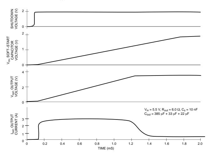
Figure 13. Typical Soft-Start Condition
