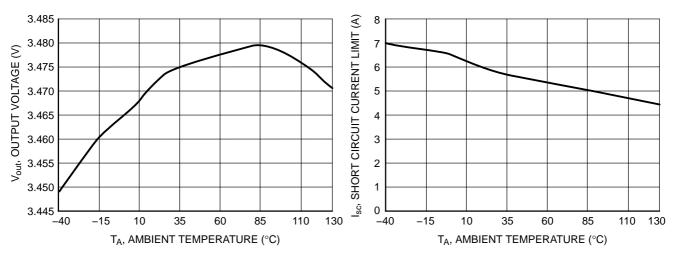
Figure 3. Output Voltage vs. Temperature
