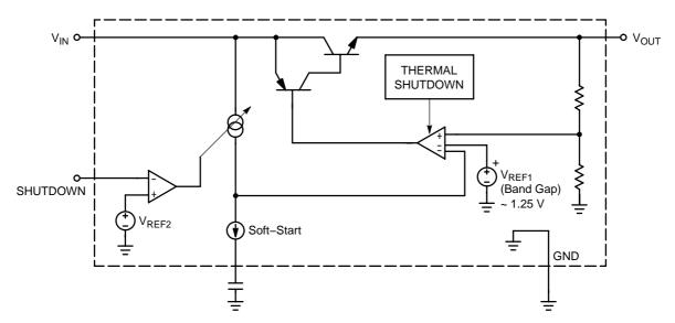
Figure 2. Simplified Block Diagram
