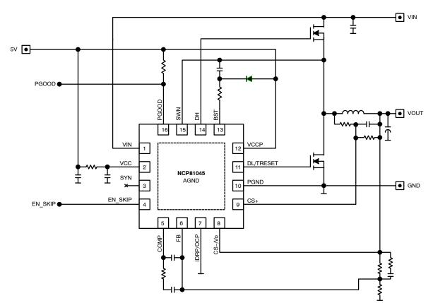
Figure 2. Typical Application Circuit (Single Device Operation)
