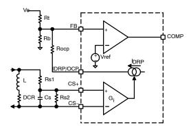
Figure 21. Configuration for AVP Function
