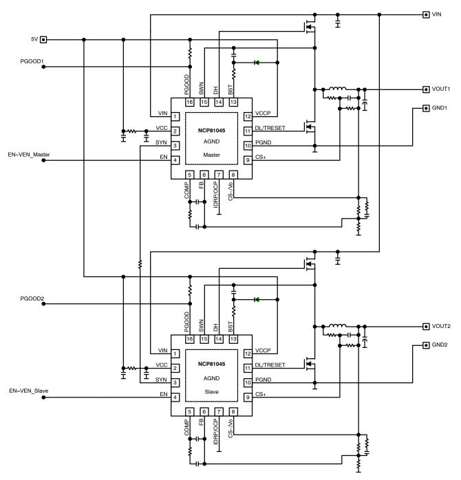
Figure 3. Typical Application Circuit (Dual Device Operation)
