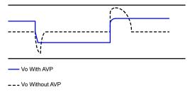
Figure 20. Adaptive Voltage Positioning
