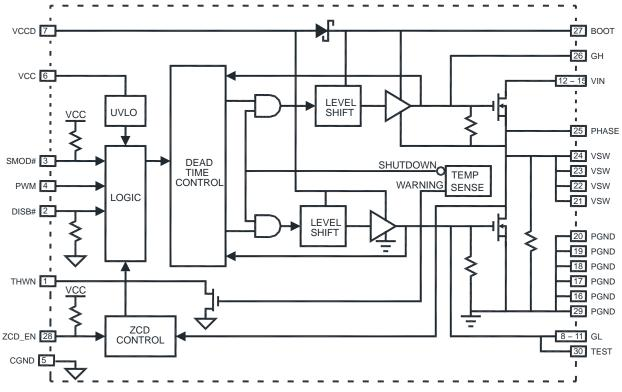
Figure 2. Block Diagram
