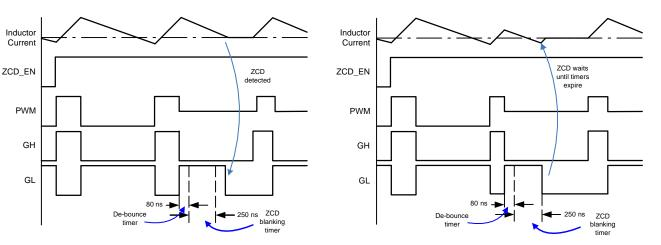
Figure 6. PWM Timing Diagram
