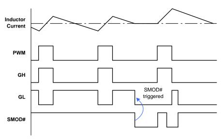
Figure 7. SMOD# Timing Diagram
