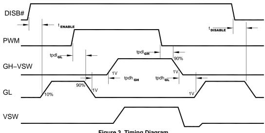
Figure 3. Timing Diagram
