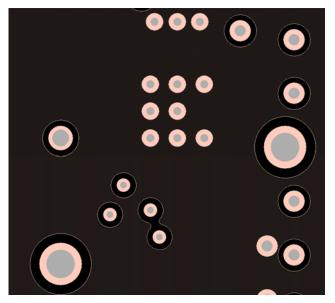
Figure 14. Layer 2 Copper Layer (Ground Plane)
