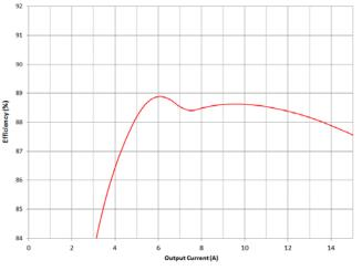
Figure 5. Efficiency – 19 V Input, 1.2 V Output, 500 kHz
