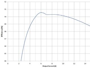
Figure 4. Efficiency – 12 V Input, 1.2 V Output, 500 kHz
