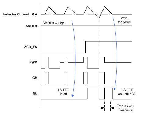
Figure 8. ZCD\_EN Timing Diagram
