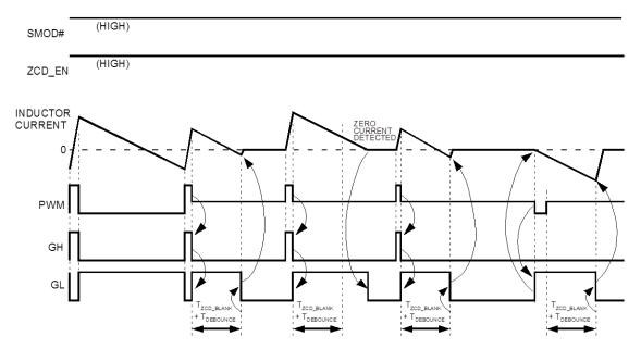
Figure 9. Timing Diagram – 3-state PWM Controller, No ZCD
