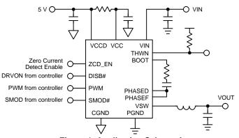
**Figure 1. Application Schematic**
