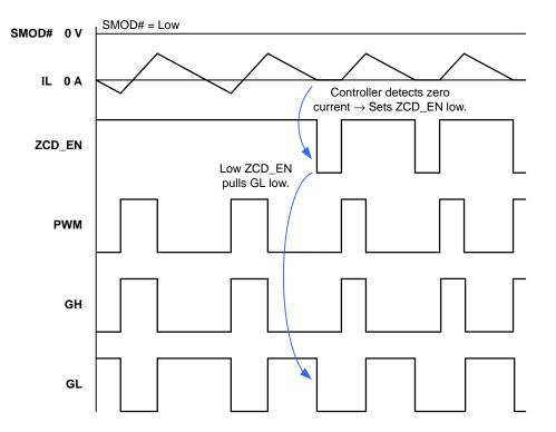
Figure 11. Timing Diagram – 2–state PWM Controller, with ZCD
