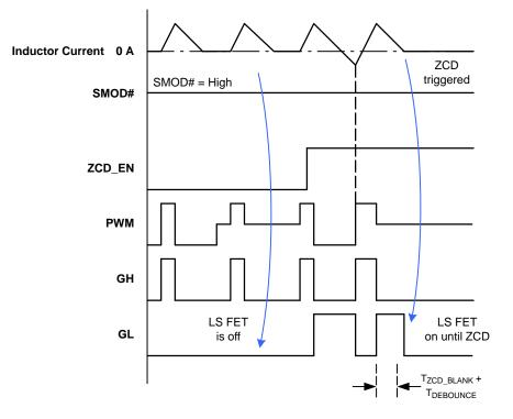
Figure 8. ZCD\_EN Timing Diagram
