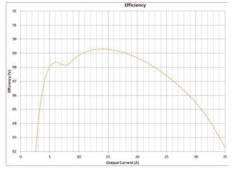
Figure 4. Efficiency – 12 V Input, 1.2 V Output, 500 kHz
