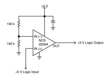
This circuit converts 5 V logic to 3 V logic. Using the NCS2220A allows for full 5 V logic swing without creating overvoltage on the 3 V logic input.
