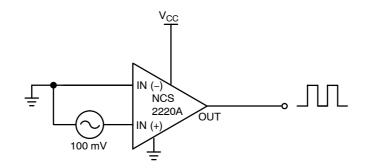
Figure 18. Zero-Crossing Detector
