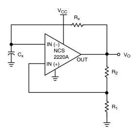
The oscillation frequency can be programmed as follows:
