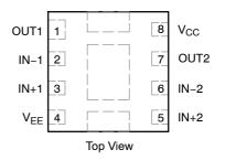
NOTE: The NCS2220A has three exposed pads on the bottom side which may be used to reduce thermal resistance by soldering to a copper heat– spreader. Electrically the exposed pads must be allowed to float.
