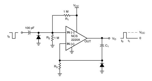
The resistor divider  $R_1$  and  $R_2$  can be used to set the magnitude of the input pulse. The pulse width is set by adjusting  $C_1$  and  $R_3.$
