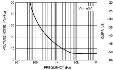
Figure 13. Input Referred Voltage Noise vs. Frequency
