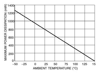
Figure 3. Power Dissipation vs. Temperature
