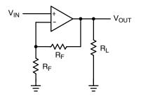
Figure 4. Typical Test Setup (A<sub>V</sub> = +2.0, R<sub>F</sub> = 1.0 k $\Omega$ , R<sub>L</sub> = 100  $\Omega$ )
