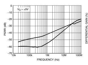
Figure 15. PSRR vs. Frequency
