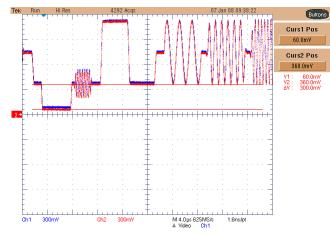
Figure 18. Multiburst Test with two 150  $\Omega$  loads
