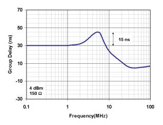
Figure 3. Group Delay vs. Frequency
