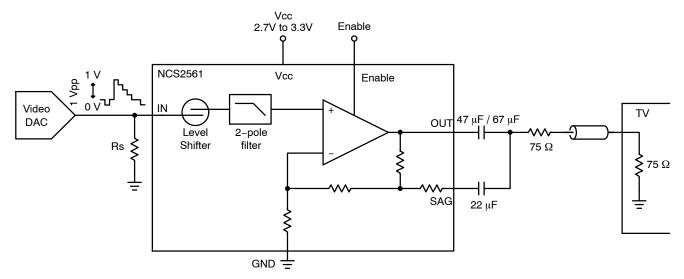
Figure 12. Sag Correction Configuration
