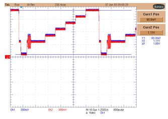
Figure 19. Linearity Test with two 150  $\Omega$  loads
