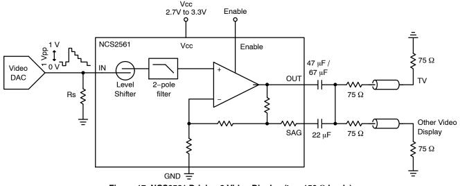
Figure 17. NCS2561 Driving 2 Video Display (two 150  $\Omega$  loads)
