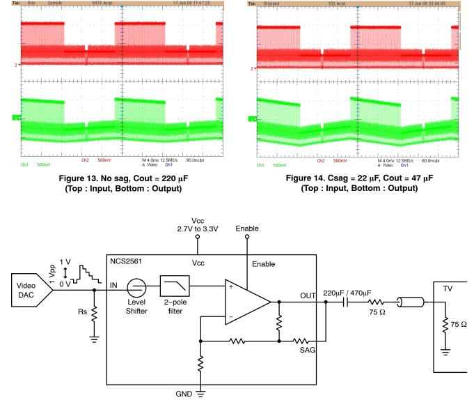
Figure 15. NCS2561 in an AC-Coupled Configuration with no sag
