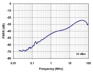
Figure 6. PSRR vs. Frequency
