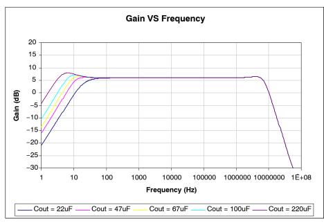
Figure 11. Simulation Results with Csag =  $22 \mu$ F and Variable Cout
