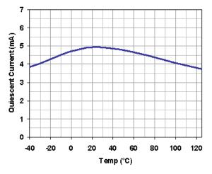
Figure 8. Quiescent Current vs. Temperature ( $V_{CC}$  = 3.0 V)
