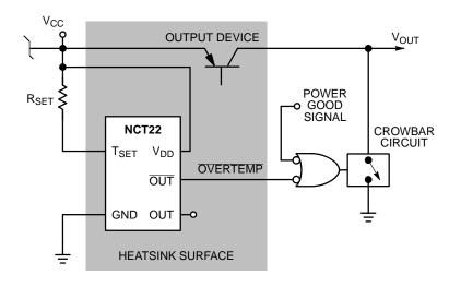
Figure 4. NCT22 Power Supply Over–Temperature Shutdown
