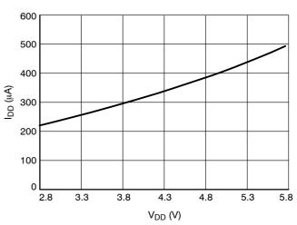
Figure 4. Supply Current vs. V<sub>DD</sub> (Temperature Conversion)
