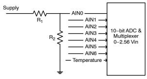
Figure 9. Resistor Divider to Attenuate the Power Supply Voltage within Required Range
