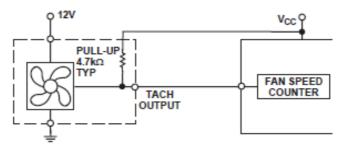
Figure 10. Fan with Tach. Pull-Up to +VCC
