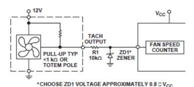
Figure 12. Fan with Strong Tach. Pull-Up to >VCC or Totem-Pole Output, Clamped with Zener and Resistor
