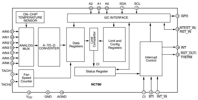
Figure 1. Functional Block Diagram of NCT80
