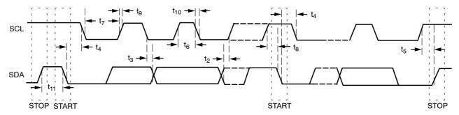
Figure 8. Serial Interface Timing
