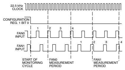
Figure 14. Fan Speed Measurement
