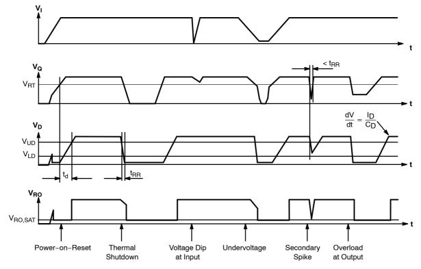
Figure 3. Reset Timing Diagram
