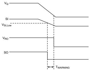
Figure 22. SO Warning Waveform Time Diagram
