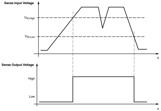
Figure 4. Sense Timing Diagram
