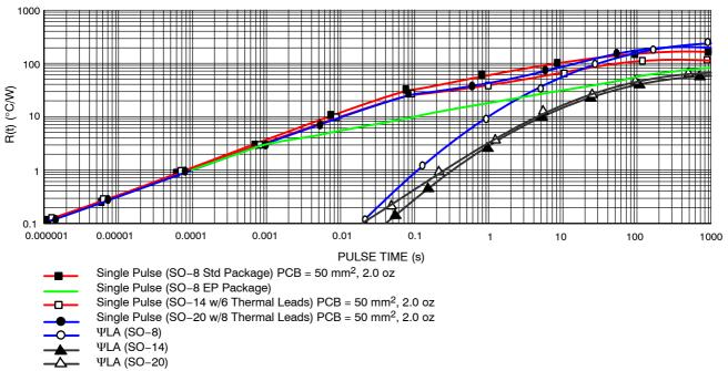
Figure 20. R(t) vs. Pulse Time
