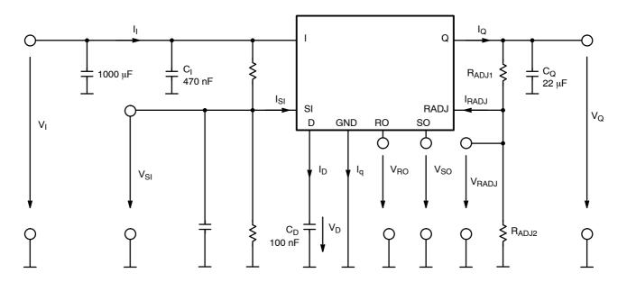
Figure 2. Measuring Circuit
