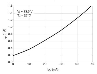
Figure 15. Current Consumption  $I_q$  vs. Output Current  $I_Q$
