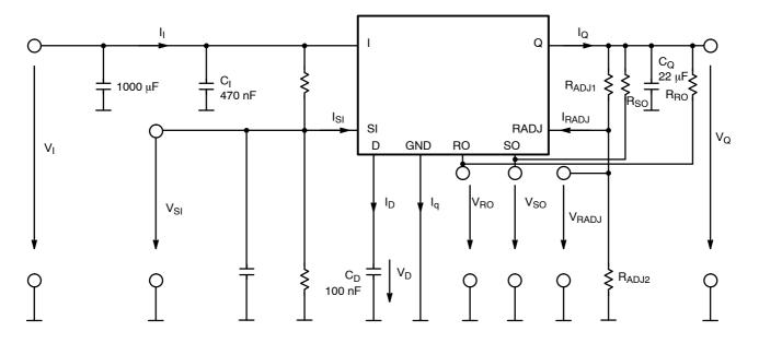
Figure 2. Measuring Circuit
