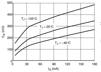
Figure 7. Drop Voltage  $V_{dr}$  vs. Output Current  $I_Q$
