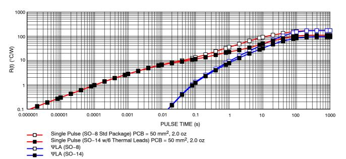
Figure 19. R(t) vs. Pulse Time
