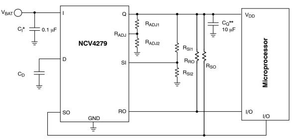
\*C<sub>I</sub> required if regulator is located far from the power supply filter.
