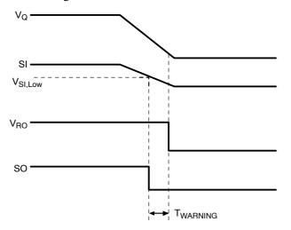
Figure 21. SO Warning Waveform Time Diagram
