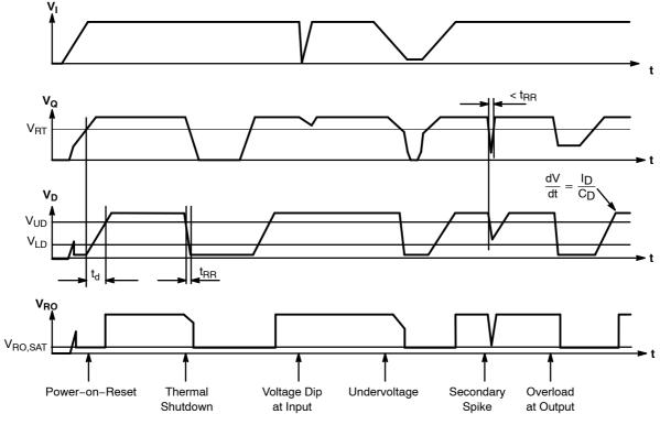
Figure 3. Reset Timing Diagram
