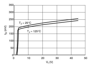
Figure 13. Output Current  ${\rm I}_{\rm Q}$  vs. Input Voltage  ${\rm V}_{\rm I}$
