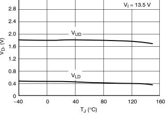
Figure 6. Switching Voltage  $V_{UD}$  and  $V_{LD}$  vs. Temperature  $T_{\rm J}$
