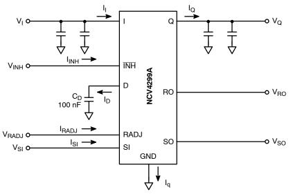
Figure 2. Measurement Circuit
