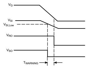
Figure 35. SO Warning Timing Waveform
