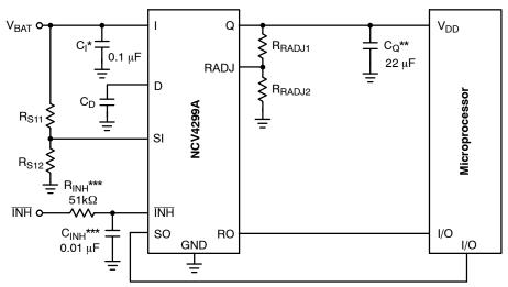
\*C<sub>1</sub> required if regulator is located far from the power supply filter.
