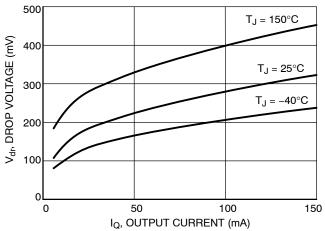
Figure 6. Drop Voltage vs. Output Current
