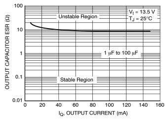
Figure 17. Output Stability vs. Output Capacitor ESR
