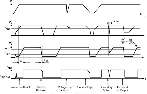
Figure 34. Reset Timing Diagram
