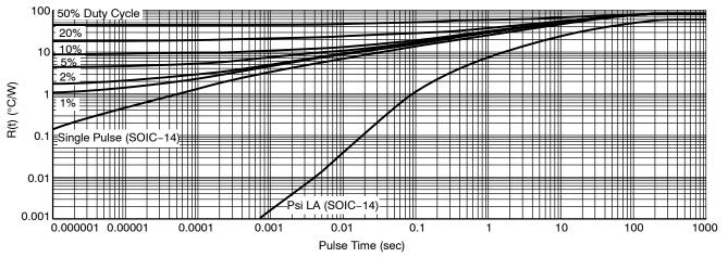
Figure 40. Transient Thermal Response Simulation to a Single Pulse with Duty Cycles Applied (Log-Log) (PCB = 250 mm<sup>2</sup> 1 oz)
