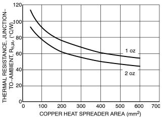
Figure 37. Thermal Resistance  $R_{\theta JA}$  vs. Copper Area
