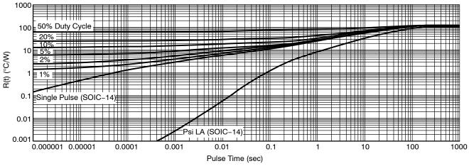
Figure 39. Transient Thermal Response Simulation to a Single Pulse with Duty Cycles Applied (Log-Log) (PCB = 50 mm<sup>2</sup> 1 oz)
