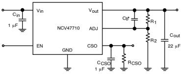
\*Required if usage of low ESR output capacitor C<sub>out</sub> is demand, see Regulator Stability Considerations section.
