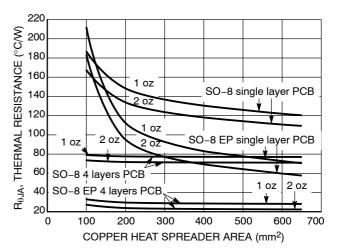
Figure 18. Thermal Resistance vs. PCB Copper Area
