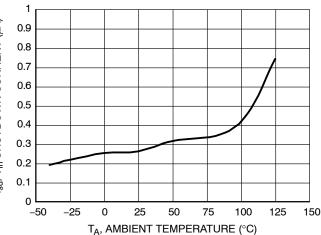
Figure 4. Standby Current vs. Temperature (EN = Low, V<sub>IN</sub> = 3.6 V)
