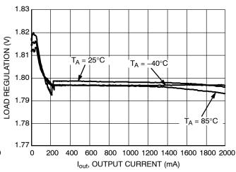
Figure 12. Load Regulation vs. Output Current and Temperature (V<sub>IN</sub> = 3.6 V, V<sub>OUT</sub> = 1.8 V).
