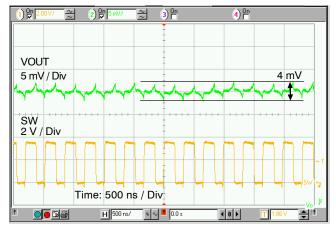
Figure 13. Output Ripple Voltage in PWM Mode ( $V_{IN}$  = 3.6 V,  $V_{OUT}$  = 1.8 V,  $I_{OUT}$  = 1 A, L=1  $\mu$ H,  $C_{OUT}$  = 10  $\mu$ F)
