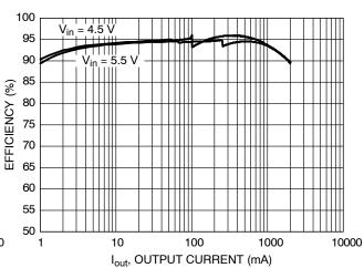
Figure 10. Efficiency vs. Output Current and Input Voltage (V<sub>OUT</sub> = 4 V , T<sub>A</sub> = 25°C)
