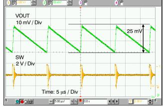
Figure 14. Output Ripple Voltage in PFM Mode ( $V_{IN}$  = 3.6 V,  $V_{OUT}$  = 1.8 V,  $I_{OUT}$  = 10 mA, L=1  $\mu$ H,  $C_{OUT}$  = 10  $\mu$ F)
