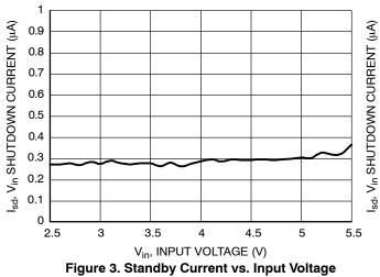
Figure 3. Standby Current vs. Input Voltage (EN = Low,  $T_A = 25$ °C)
