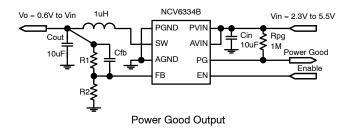
Figure 1. Typical Application Circuits
