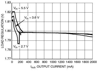
Figure 11. Load Regulation vs. Output Current and Input Voltage (V<sub>OUT</sub> = 1.8 V, T<sub>A</sub> = 25°C)
