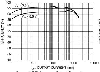
Figure 9. Efficiency vs. Output Current and Input Voltage (V<sub>OUT</sub> = 3.3 V, T<sub>A</sub> = 25°C)
