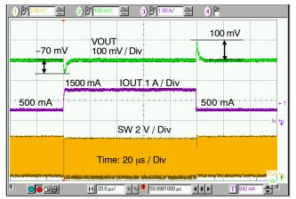
Figure 15. Load Transient Response (V<sub>IN</sub> = 3.6 V, V<sub>OUT</sub> = 1.8 V, I<sub>OUT</sub> = 500 mA to 1500 mA, L = 1  $\mu$ H, C<sub>OUT</sub> = 10  $\mu$ F)
