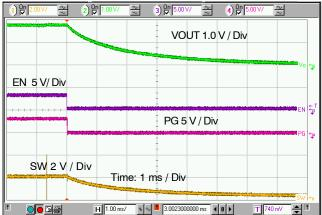
Figure 17. Power Up Sequence and Power Good (V<sub>IN</sub> = 3.6 V, V<sub>OUT</sub> = 1.8 V, I<sub>OUT</sub> = 0 A, L = 1  $\mu$ H, C<sub>OUT</sub> = 10  $\mu$ F)
