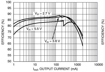
Figure 7. Efficiency vs. Output Current and Input Voltage (V<sub>OUT</sub> = 1.05 V, T<sub>A</sub> = 25°C)
