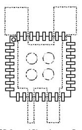
Figure 3. Example of QFN32 PCB Ground Plane Layout. Preferred layout at top and bottom connected with through-hole filled vias
