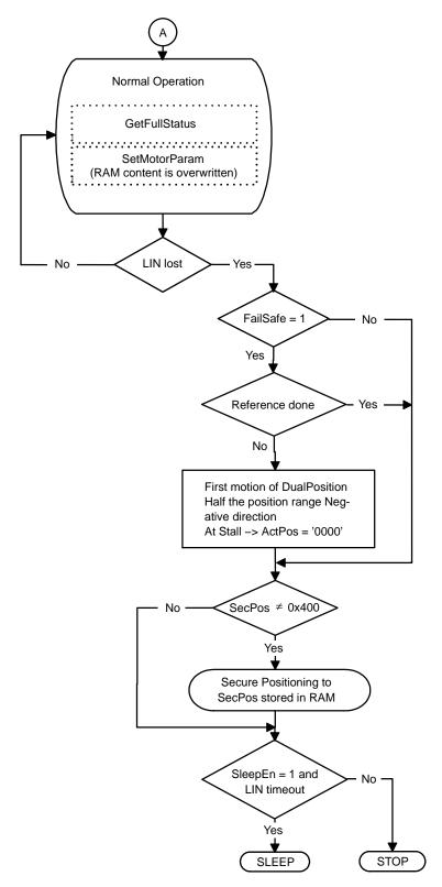
Figure 24. LIN Lost During Normal Operation
