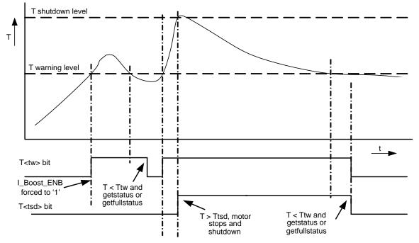
Figure 14. Illustration of Thermal Management Situation
