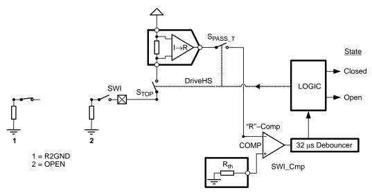
Figure 11. Simplified Schematic Diagram of the SWI Comparator
