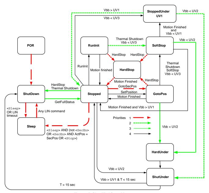
Figure 15. Simplified State Diagram
