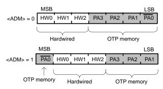
Figure 22. Combination of OTP and Hardwired address bits in function of ADM (Address Mode)
