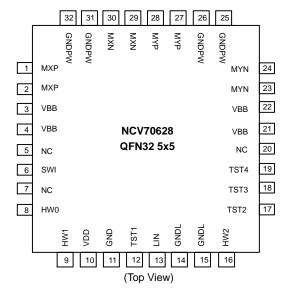
Figure 2. Pinout Diagram
