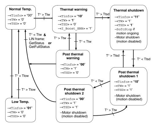
Figure 13. State Diagram Temperature Management
