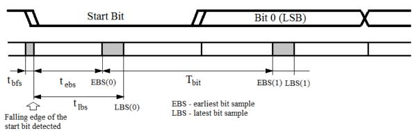
Figure 21. Bit Sample Timing
