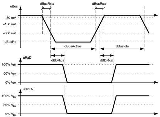
Figure 13. Parameters of Bus Activity Detection
