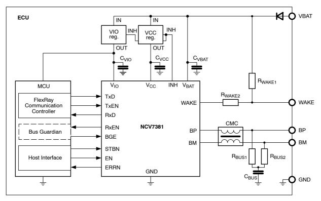
Figure 2. Application Diagram
