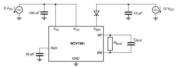
Figure 17. Test Setup for Dynamic Characteristics
