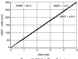
Figure 16. INH Not\_Sleep Output Characteristic
