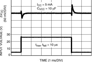
Figure 10. Line Transient Response (Vbb 5 V to 26 V)
