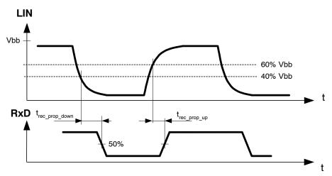
Figure 26. LIN Receiver Timing
