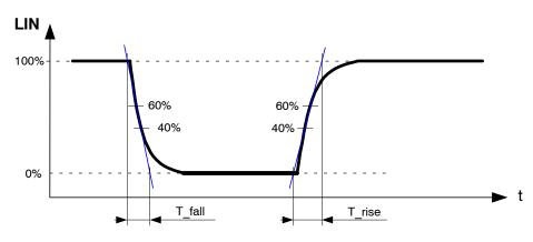
Figure 25. LIN Transmitter Rising and Falling Times
