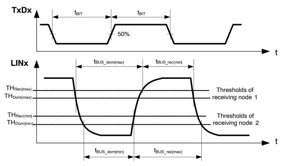
Figure 5. LIN Transmitter Duty Cycle
