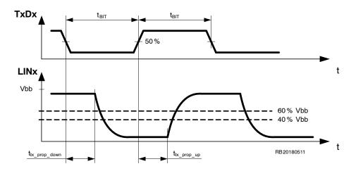
Figure 7. LIN Transmitter Timing
