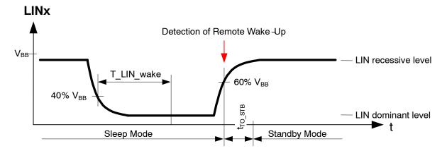
Figure 4. Remote (LIN) Wake-up Detection
