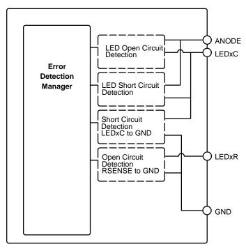
Figure 7. Short Circuit and Open Circuit Detection
