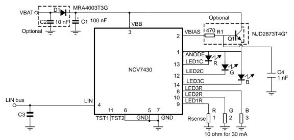
Figure 3. Typical Application with Ballast Transistor
