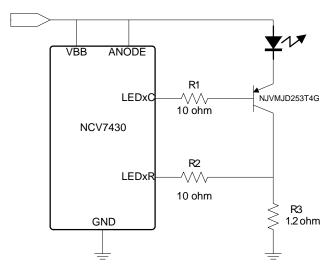
Figure 12. Using the NCV7430 with Higher Current LEDs
