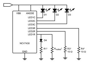
Figure 13. External Temperature Compensation
