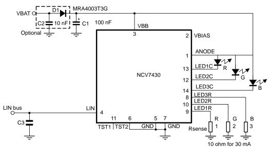
Figure 4. Typical Application without Ballast Transistor
