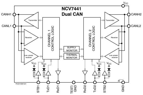
Figure 1. NCV7441 Dual CAN: Block Diagram
