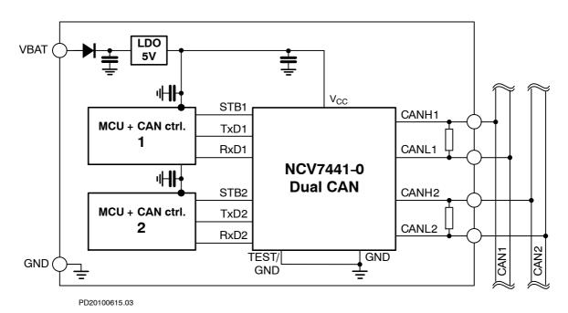
Figure 2. NCV7441 Dual CAN: Example Application Diagram
