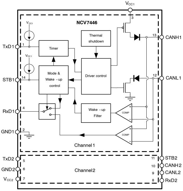
Figure 1. NCV7446 Block Diagram
