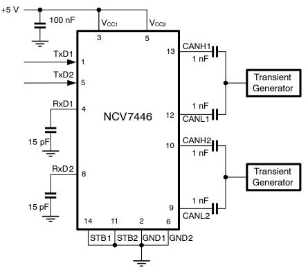
Figure 5. Test Circuit for Automotive Transients
