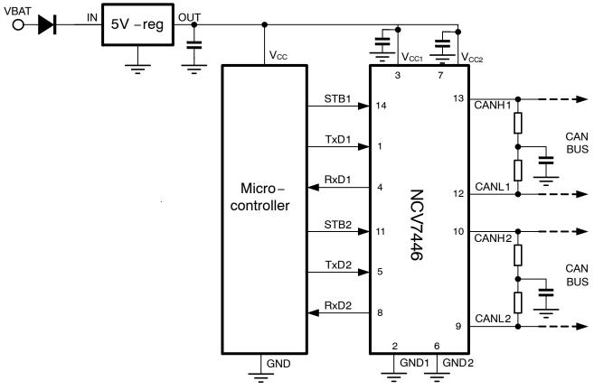
Figure 2. NCV7446 Application Diagram
