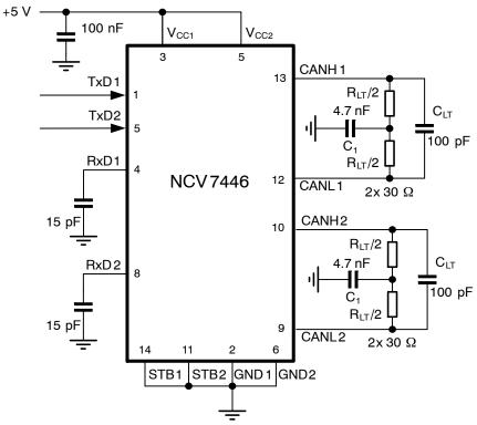
Figure 6. Test Circuit for Timing Characteristics
