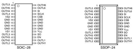
Figure 2. Pin Connection
