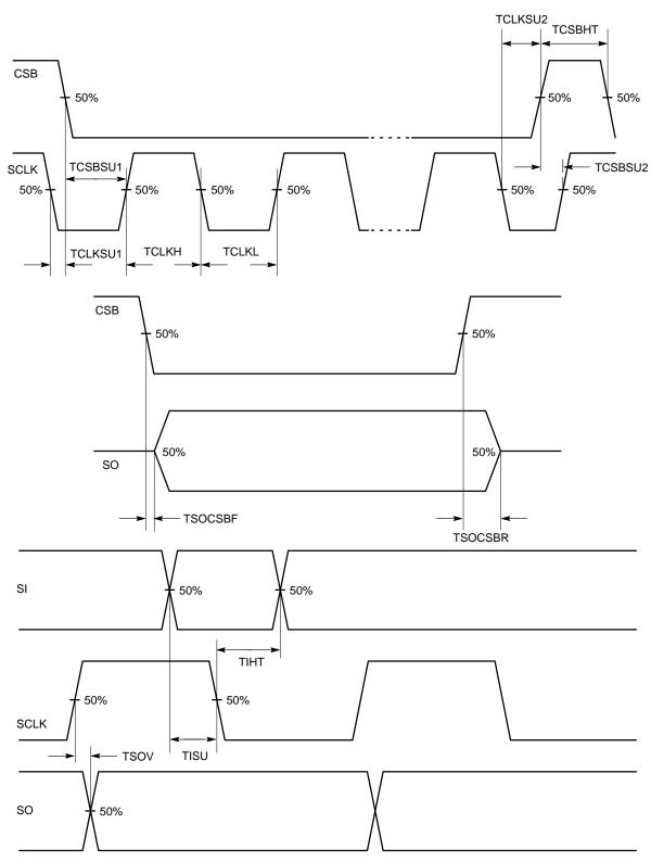
Figure 3. SPI Timing Diagram
