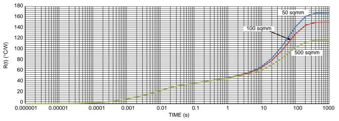
Figure 17. SSOP24 Narrow Body Exposed Pad Single Pulse Heating Curve
