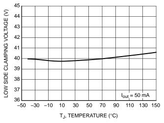
Figure 11. Low-Side Clamping Voltage vs. Temperature
