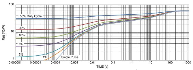
Figure 16. SOIC 28-Lead Thermal Duty Cycle Curve on 986 mm<sup>2</sup> Spreader Test Board
