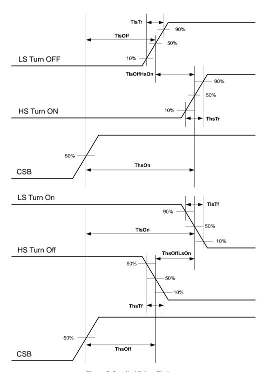
Figure 5. Detailed Driver Timing
