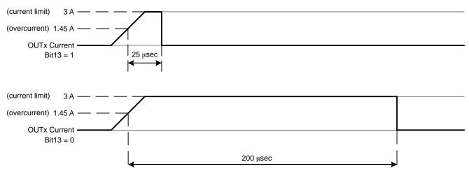
**Figure 6. Output Current Shutdown Control**
