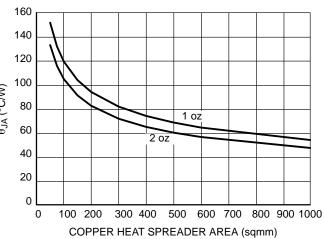
Figure 14. SSOP24 Narrow Body Exposed Pad  $\theta_{JA}$  vs. Copper Spreader Area
