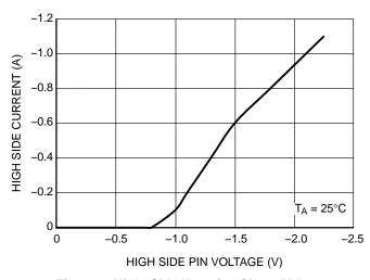
Figure 9. High-Side Negative Clamp Voltage vs. Reverse Current
