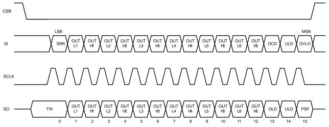
Figure 4. SPI Communication Frame Format
