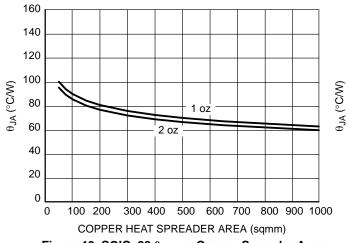
Figure 13. SOIC–28  $\theta_{\text{JA}}$  vs. Copper Spreader Area
