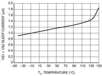
Figure 12. VS1 + VS2 Sleep Current vs. Temperature
