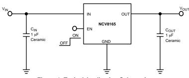
**Figure 1. Typical Application Schematics**
