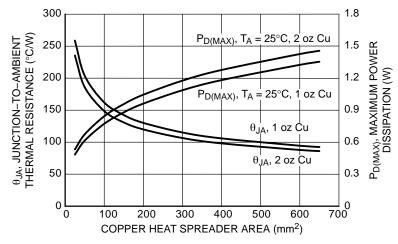
Figure 22.  $\theta_{JA}$  and  $P_{D(MAX)}$  vs. Copper Area (DFNW8)
