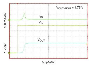
Figure 19. Turn-ON - V<sub>IN</sub> Driven (fast)
