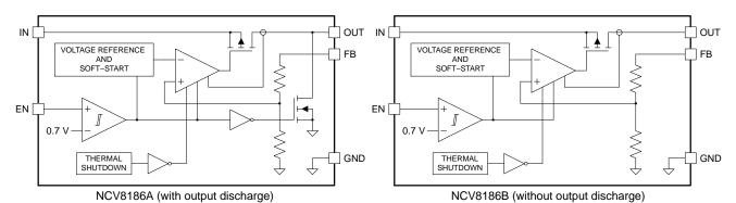
Figure 2. Internal Block Diagram
