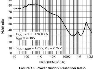
Figure 16. Power Supply Rejection Ratio
