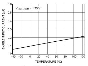
Figure 15. Enable Input Current vs. **Temperature**
