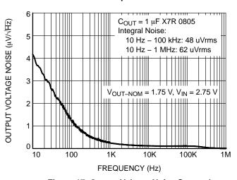
Figure 17. Output Voltage Noise Spectral **Density**
