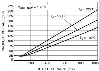
Figure 5. Load Regulation vs. Temperature
