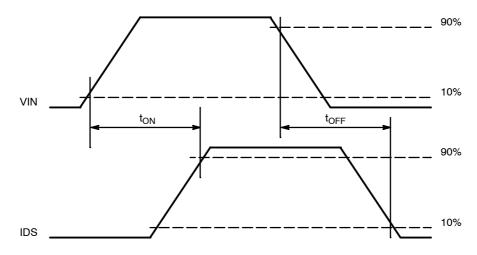
Figure 23. Resistive Load Switching Waveforms
