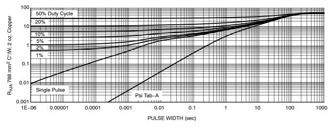
Figure 21. Transient Thermal Resistance
