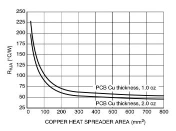
Figure 20.  $R_{\theta JA}$  vs. Copper Area
