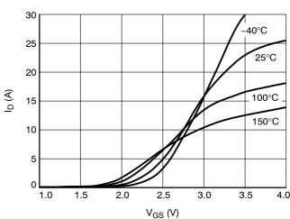
Figure 7. Transfer Characteristics (V<sub>DS</sub> = 10 V)
