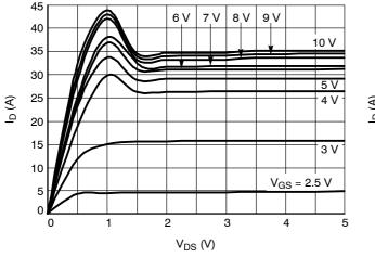
Figure 6. On-state Output Characteristics at 25°C
