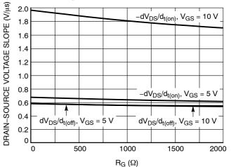
Figure 18. Resistive Load Switching Time vs. Gate Resistance ( $V_{DD} = 25 \text{ V}$ ,  $I_D = 5 \text{ A}$ )
