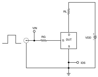
Figure 22. Resistive Load Switching Test Circuit
