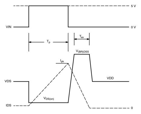
Figure 25. Inductive Load Switching Waveforms
