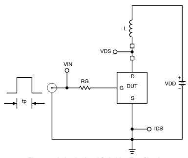
Figure 24. Inductive Load Switching Test Circuit
