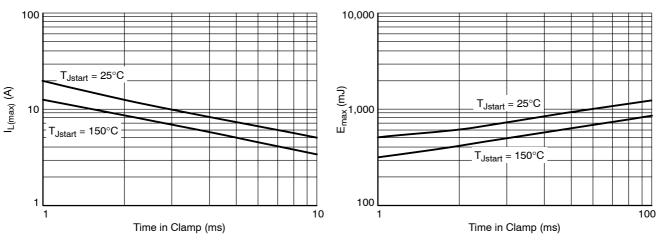
Figure 4. Single Pulse Maximum Inductive Switch-off Current vs. Time in Clamp
