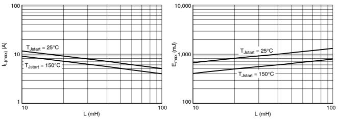
Figure 2. Single Pulse Maximum Switch-off Current vs. Load Inductance
