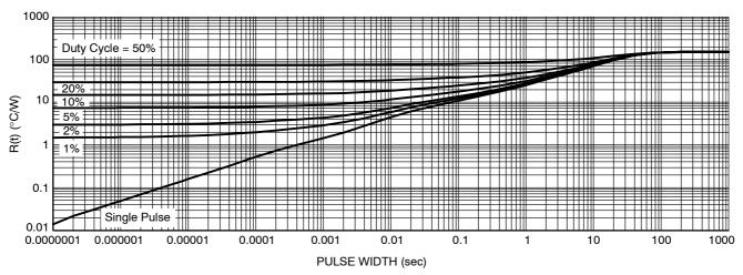
Figure 20. Transient Thermal Resistance
