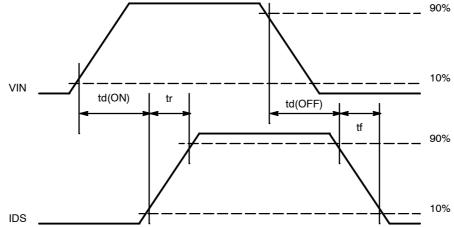
Figure 22. Resistive Load Switching Waveforms
