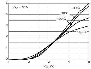
Figure 7. Transfer Characteristics
