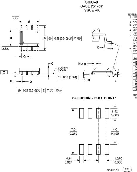
1. DIMENSIONING AND TOLERANCING PER ANSI Y14.5M, 1982.
