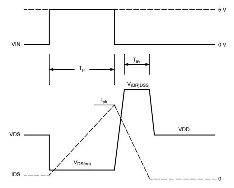
Figure 24. Inductive Load Switching Waveforms
