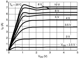
Figure 6. On-state Output Characteristics
