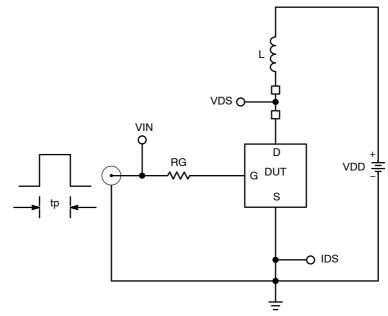
Figure 23. Inductive Load Switching Test Circuit
