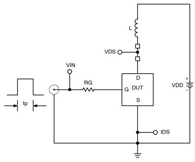
Figure 4. Inductive Load Switching Test Circuit
