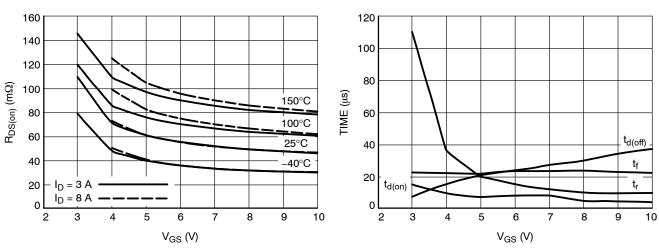
Figure 8. R<sub>DS(on)</sub> vs. Gate Voltage
