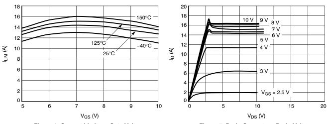
Figure 6. Current Limit vs. Gate Voltage
