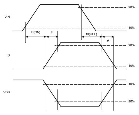
Figure 3. Resistive Load Switching Waveforms
