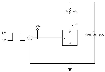
Figure 2. Resistive Load Switching Test Circuit
