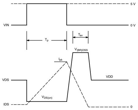
Figure 5. Inductive Load Switching Waveforms
