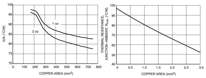
Figure 22. SOIC 16-Lead  $\theta$ JA as a Function of the Pad Copper Area Including Traces, Board Material
