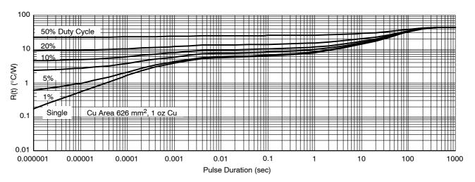
Figure 31. D<sup>2</sup>PAK 7-Lead Thermal Duty Cycle Curves on 1" Spreader Test Board
