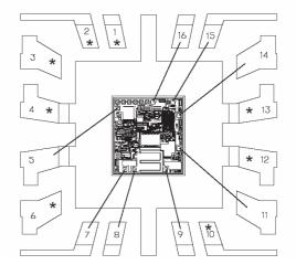
Figure 21. Internal Construction of the Package (notice pins 4, 5 and 12, 13 are connected to flag)
