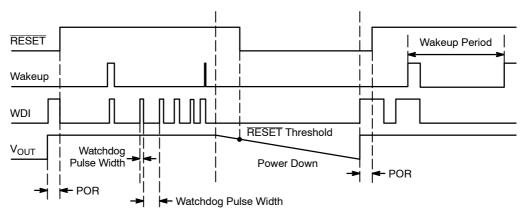
Figure 5. Power Down and Restart Sequence
