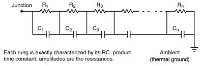
Figure 39. Non-Grounded Capacitor Thermal Ladder ("Foster" Ladder)
