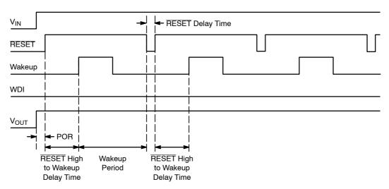
Figure 4. Error Condition: Watchdog Remains Low and a RESET Is Issued
