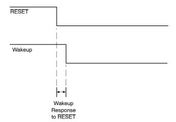
Figure 18. Wakeup Response to RESET (Low Voltage)
