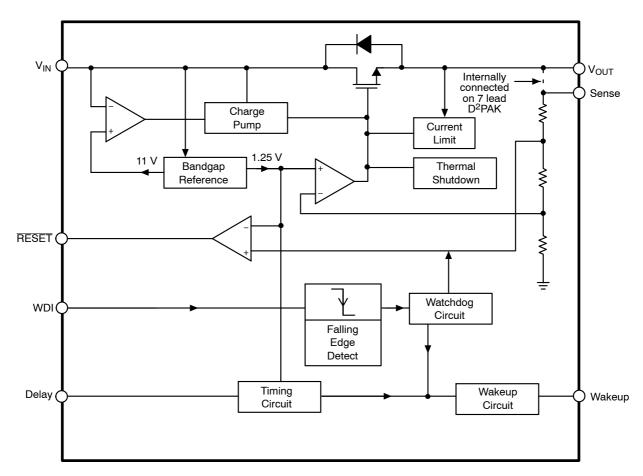
Figure 2. Block Diagram
