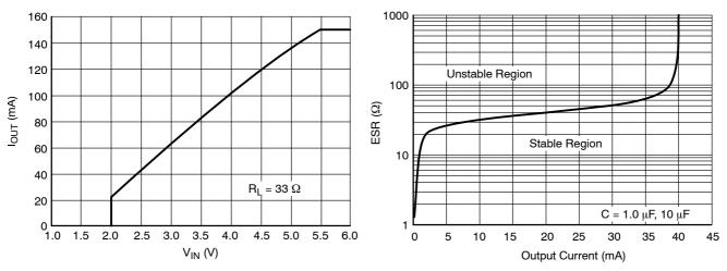
Figure 14. Output Current vs Input Voltage
