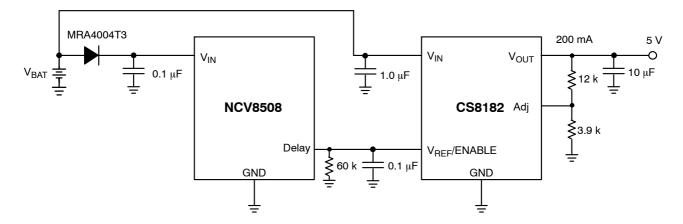
Figure 16. Application Circuit
