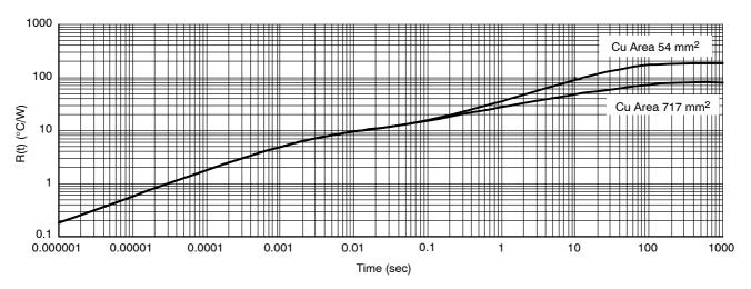
Figure 36. SOIC 8-Lead EP Single Pulse Heating Curve
