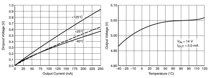
Figure 12. Dropout Voltage vs Output Current
