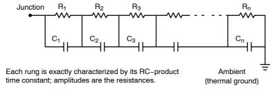
Figure 27. Non-Grounded Capacitor Thermal Ladder ("Foster" Ladder)
