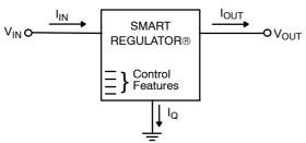
Figure 40. Single Output Regulator with Key Performance Parameters Labeled
