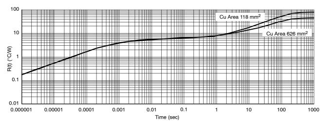
Figure 30. D<sup>2</sup>PAK 7-Lead Single Pulse Heating Curve
