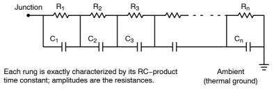
Figure 33. Non-Grounded Capacitor Thermal Ladder ("Foster" Ladder)
