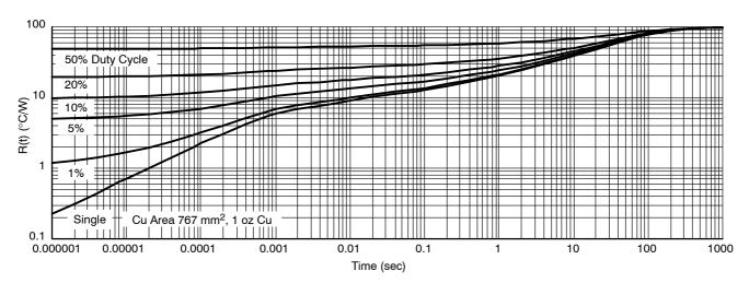
Figure 25. SOIC 16-Lead Thermal Duty Cycle Curves on 1" Spreader Test Board
