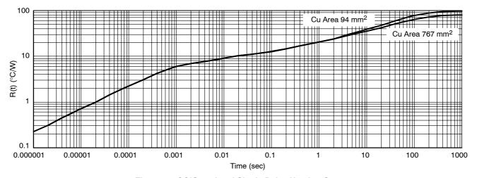
Figure 24. SOIC 16-Lead Single Pulse Heating Curve
