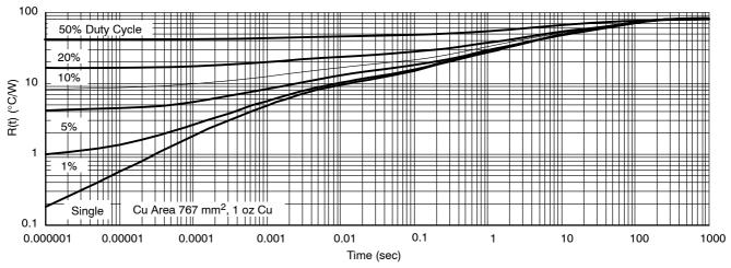
Figure 37. SOIC 8-Lead Thermal Duty Cycle Curves on 1" Spreader Test Board
