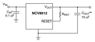
\*C<sub>IN</sub> required if regulator is located far from the power supply filter. \*\*C<sub>OUT</sub> required for stability. Capacitor must operate at minimum temperature expected.
