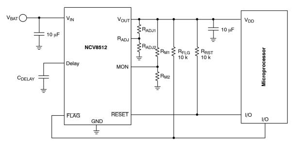
Figure 1. Application Diagram
