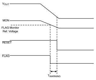
Figure 14. FLAG Monitor Circuit Waveform
