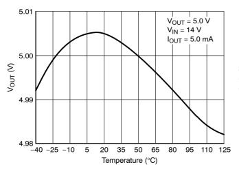
Figure 2. Output Voltage vs. Temperature
