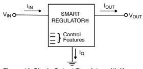
Figure 16. Single Output Regulator with Key Performance Parameters Labeled
