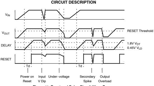
Figure 11. Reset and Delay Circuit Wave Forms
