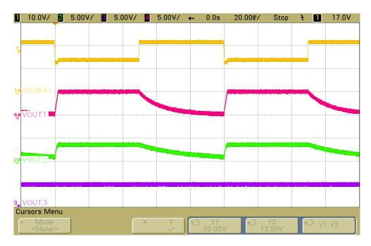
Figure 34. Output Response to OVS - VBAT-MON tied to ASO-RAIL
