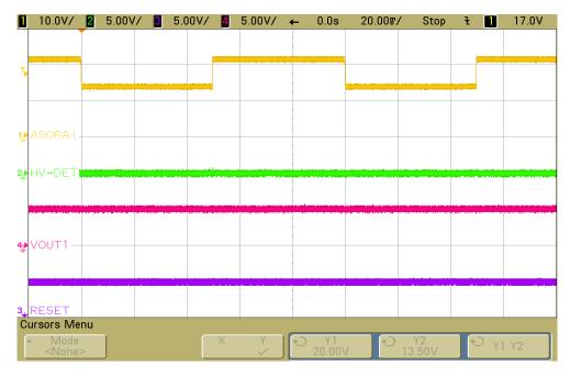
Figure 31. HV-DET Response to High Voltage - VBAT-MON Left Open
