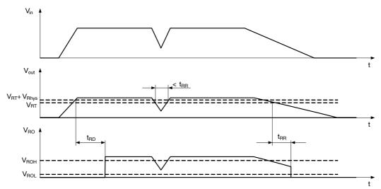
Figure 24. Reset Function and Timing Diagram
