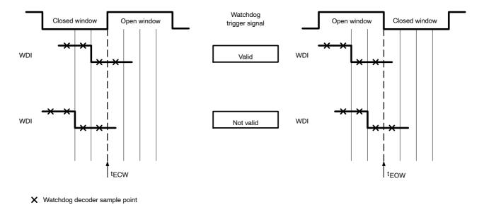
Figure 27. Valid WDI trigger signal
