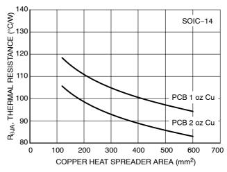
Figure 28. Thermal Resistance vs PCB Copper Area
