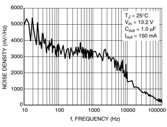
Figure 18. Noise vs. Frequency
