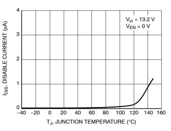
Figure 19. Disable Current vs Temperature
