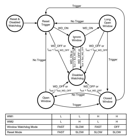
Figure 25. Window Watchdog State Diagram, Watchdog and Reset Modes
