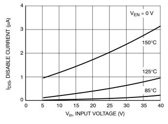
Figure 20. Disable Current vs. Input Voltage
