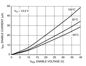
Figure 21. Enable Current vs. Enable Voltage
