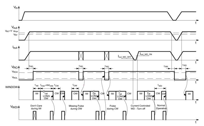
Figure 26. Window Watchdog Signal Diagram
