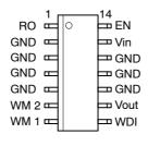
Figure 3. Pin Connections (Top View)
