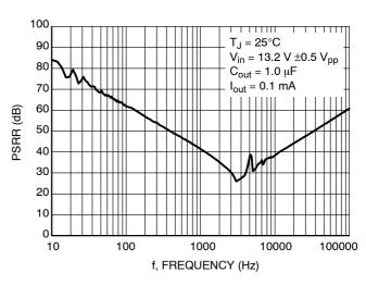
Figure 17. PSRR vs. Frequency
