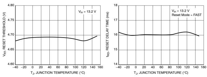
Figure 22. Reset Threshold vs Temperature
