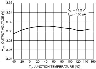
Figure 8. Output Voltage vs. Temperature (3.3 V Option)
