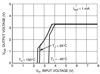
Figure 10. Output Voltage vs. Input Voltage (3.3 V Option)
