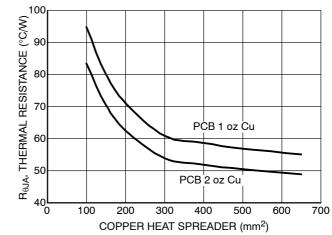
Figure 34. Thermal Resistance vs. PCB Copper Area (D2PAK-5)
