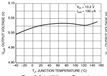
Figure 7. Output Voltage vs. Temperature (5 V Option)
