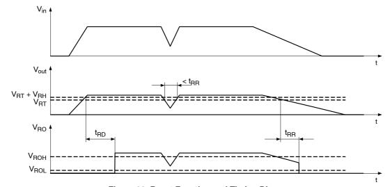
Figure 33. Reset Function and Timing Diagram
