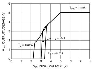
Figure 9. Output Voltage vs. Input Voltage (5 V Option)
