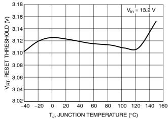
Figure 30. Reset Threshold vs. Temperature (5 V Option)
