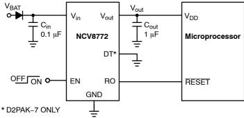
Figure 1. Typical Application Schematic
