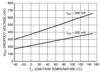
Figure 12. Dropout vs. Temperature (5 V Option)
