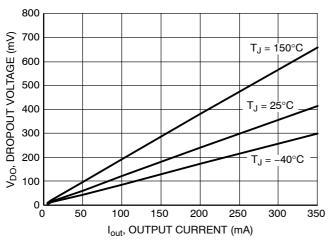
Figure 11. Dropout vs. Output Current (5 V Option)
