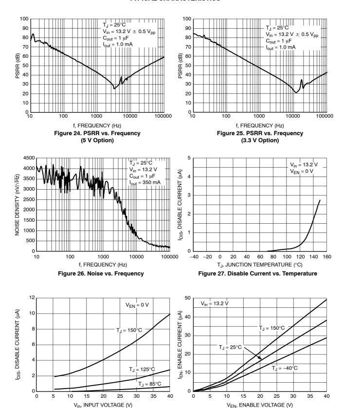
Figure 28. Disable Current vs. Input Voltage
