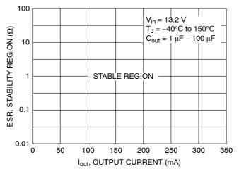
Figure 17. C<sub>out</sub> ESR Stability Region vs. Output Current
