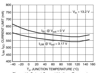
Figure 16. Output Current Limit vs. Temperature (3.3 V Option)
