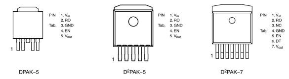
Figure 3. Pin Connections
