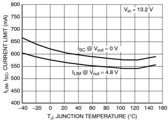
Figure 15. Output Current Limit vs. Temperature (5 V Option)
