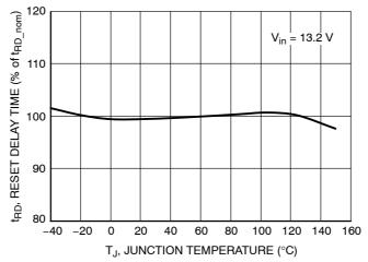
Figure 32. Reset Delay Time vs. Temperature
