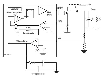
Figure 11. Current Mode Control Schematic
