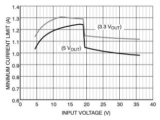
Figure 26. NCV890100 Load Current Capability with 4.7 µH Inductor
