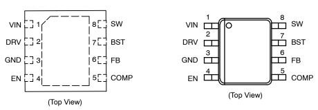
Figure 3. Pin Connections
