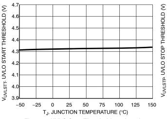
Figure 6. UVLO Start Threshold vs. Junction Temperature
