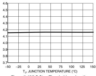
Figure 7. UVLO Stop Threshold vs. Junction Temperature
