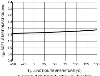
Figure 8. Soft-Start Duration vs. Junction Temperature
