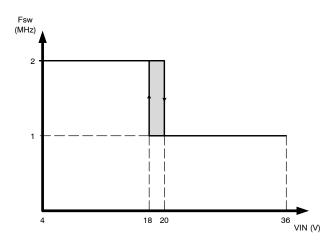
Figure 25. NCV890100 Switching Frequency Reduction at High Input Voltage
