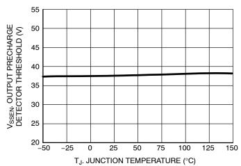
Figure 24. Output Precharge Detector Threshold vs. Junction Temperature
