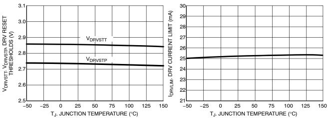
Figure 22. DRV Reset Threshold vs. Junction Temperature
