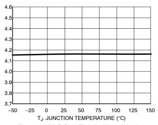
Figure 7. UVLO Stop Threshold vs. Junction Temperature
