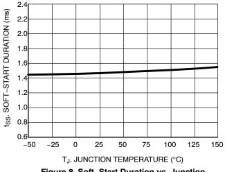
Figure 8. Soft-Start Duration vs. Junction Temperature
