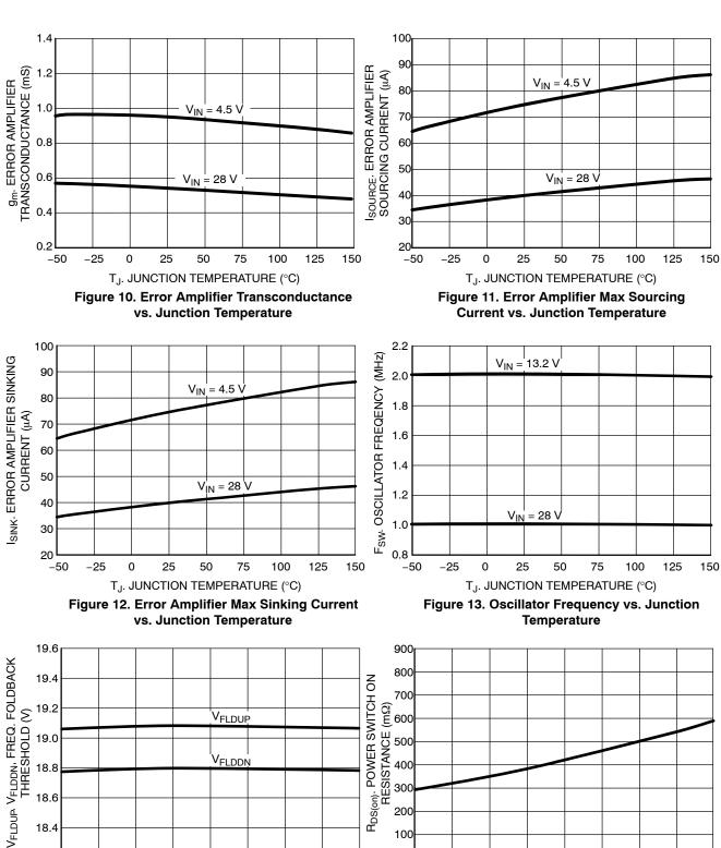
T<sub>.I</sub>. JUNCTION TEMPERATURE (°C) Figure 14. Rising Frequency Foldback Threshold vs. Junction Temperature
