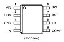
Figure 3. Pin Connections
