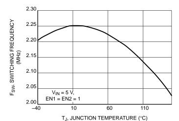
Figure 11. Switching Frequency vs.
