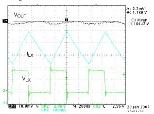
Figure 12. PWM Switching Waveforms ( $V_{IN} = 3.6 \text{ V}$ ,  $V_{OUT} = 1.2 \text{ V}$ ,  $I_{OUT} = 600 \text{ mA}$ , Temp = 25°C)
