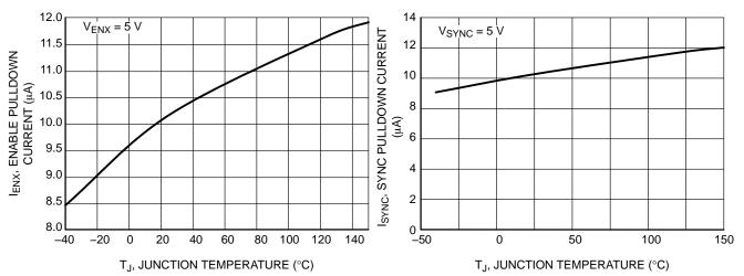
Figure 9. Enable Pulldown Current vs. Temperature
