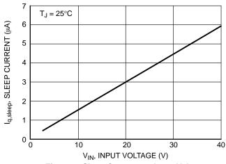
Figure 2. Sleep Current vs. Input Voltage
