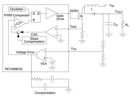
Figure 12. Boost Current Mode Schematic
