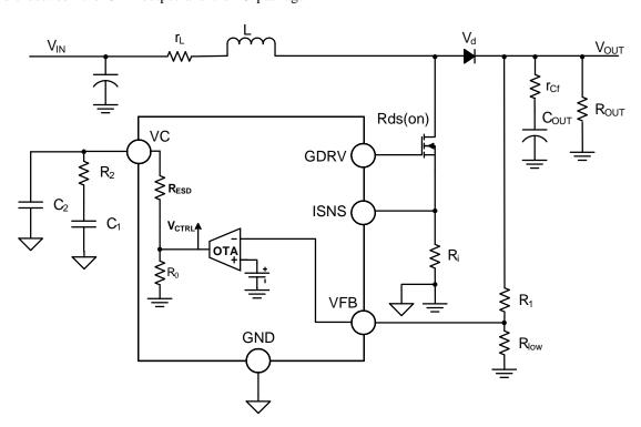
Figure 13. NCV898032 Boost Converter OTA and Compensation
