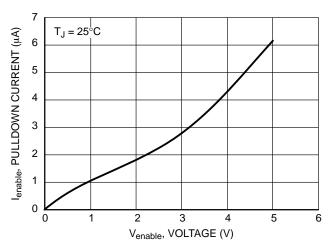
Figure 8. Enable Pulldown Current vs. Voltage
