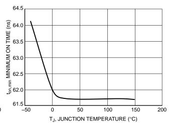
Figure 5. Minimum On Time vs. Temperature
