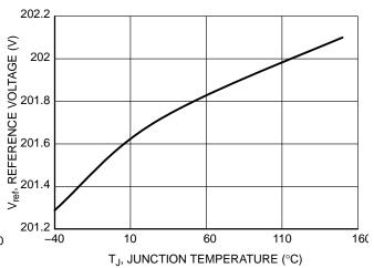
Figure 7. Reference Voltage vs. Temperature
