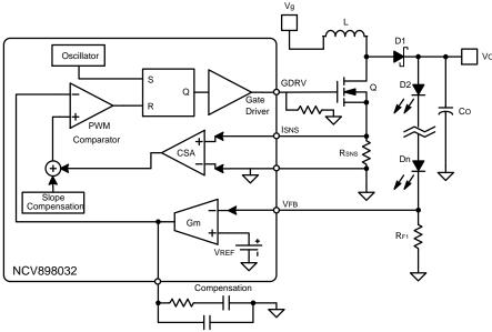
Figure 10. Current Mode Control Schematic
