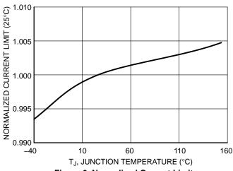
Figure 6. Normalized Current Limit vs. Temperature
