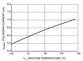
Figure 9. Enable Pulldown Current vs. Temperature
