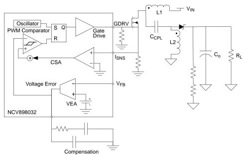
Figure 11. SEPIC Current Mode Schematic
