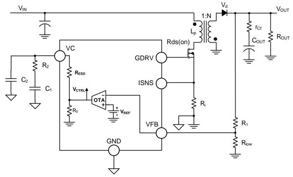
Figure 14. NCV898032 Flyback Converter OTA and Compensation
