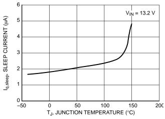
Figure 3. Sleep Current vs. Temperature
