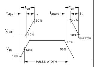
Figure 12. Switching Waveforms.
