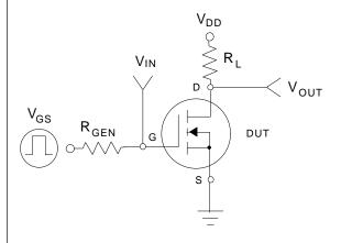
Figure 11. Switching Test Circuit.
