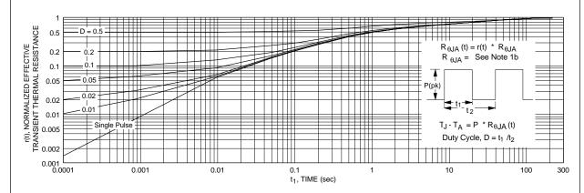
Figure 17. Transient Thermal Response Curve.
