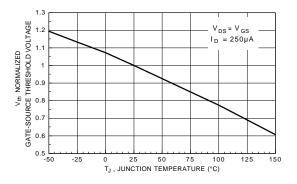
Figure 6. Gate Threshold Variation with Temperature.
