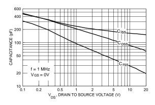
Figure 9. Capacitance Characteristics.
