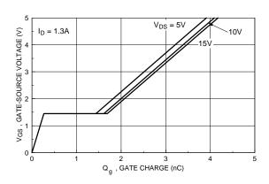
Figure 10. Gate Charge Characteristics.
