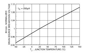
Figure 7. Breakdown Voltage Variation with Temperature.
