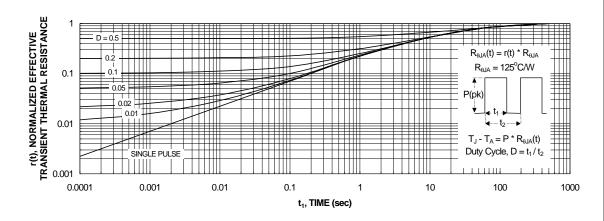
Figure 11. Transient Thermal Response Curve.
