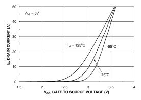
Figure 5. Transfer Characteristics.
