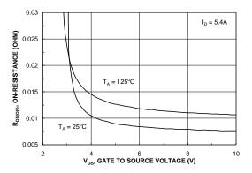
Figure 4. On-Resistance Variation with Gate-to-Source Voltage.
