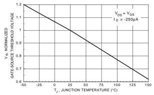
Figure 6. Gate Threshold Variation with Temperature.
