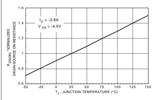
Figure 3. On-Resistance Variation with Temperature.
