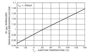
Figure 7. Breakdown Voltage Variation with Temperature.
