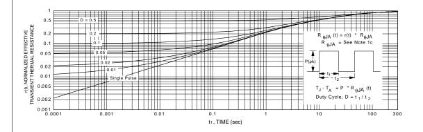
Figure 15. Transient Thermal Response Curve.
