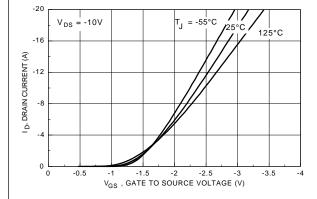
Figure 5. Transfer Characteristics.
