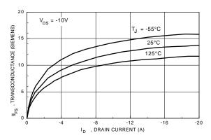
Figure 11. Transconductance Variation with Drain Current and Temperature.
