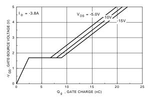
Figure 10. Gate Charge Characteristics.
