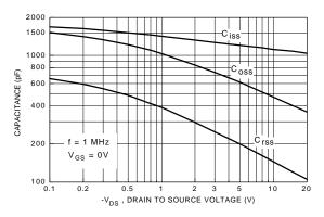
Figure 9. Capacitance Characteristics.
